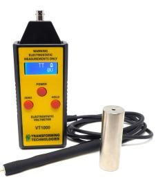
hand-held probe is included in its standard configuration, which can be used to test human walking voltage.
